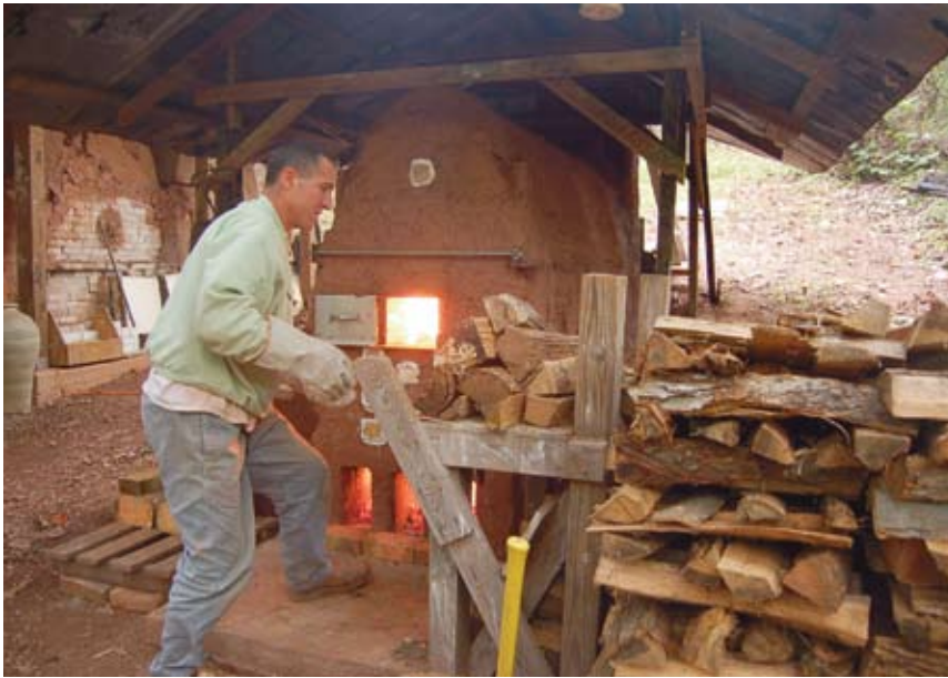
John Thies stokes the 24-cubic-foot Manabigama from the front.
